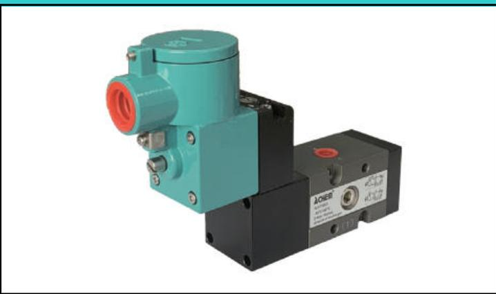
The multi-function flameproof solenoid valves of aluminum is available with both Namur connection and In-line connection and also is easily switched between 3/2 and 5/2 for the same valve body. The flow rate of the valve is relatively large, and the air port is BSPP1/4" or NPT1/4". Armed with aluminum enclosure coil, this solenoid valve is excellent for being used in corrosive and hazardous area(Class I Zone 0 AEx ia IIC T6 Ga)
